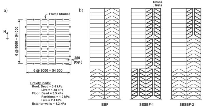
Figure 3 Floor plane view and elevation view of the lateral force resisting system: a) floor plane view and loading condition; b) structural configurations studied.
