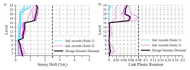
Figure 7 Peak storey drift profiles and peak link inelastic rotations for the SESBF-1: a) Peak storey drift profiles; b) Peak link inelastic rotation profiles.
