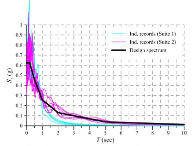
Figure 5 5% damped acceleration spectra of the scaled ground motion records.
