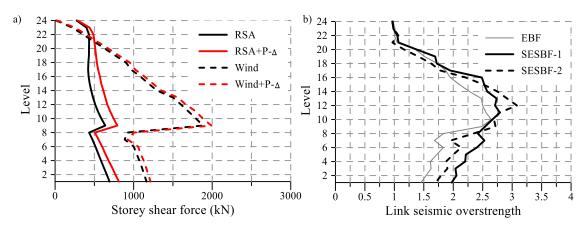
Figure 4 a) EBF design factored storey shears (/braced bay); b) Link seismic overstrength
