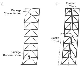
Figure 2. Deformed shape of an 8-storey structure: a) Conventional EBF; b) SESBF with 2 four-storey trussed spine segments.
