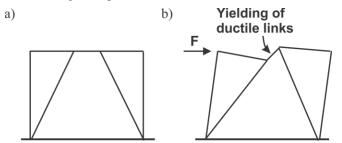
Figure 1 Eccentrically braced frame (EBF) system: a) Typical configuration; b) Intended yielding mechanism.
