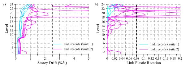
Figure 6 Peak storey drift profiles and peak link inelastic rotations for the conventional EBF: a) Peak storey drift profiles; b) Peak link inelastic rotation profiles.
