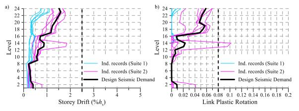
Figure 8 Peak storey drift profiles and peak link inelastic rotations for the SESBF-2: a) Peak storey drift profiles; b) Peak link inelastic rotation profiles.
